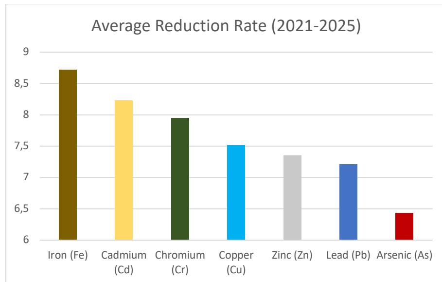
At the end of the experiment, results indicated that Iron (Fe) exhibited the highest average reduction rate at 8.2 suggesting it was the most readily sequestered or stabilized heavy metal, followed by Cadmium, Chromium, Copper, Zinc and Lead, while Arsenic (As) showed the lowest overall reduction rate.
